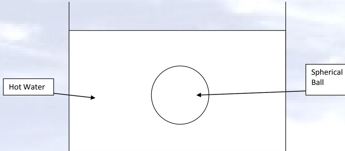
$$\frac{k}{r^2} \frac{\partial}{\partial r} \left( r^2 \frac{\partial T}{\partial r} \right) + \frac{k}{r^2 \sin \theta} \frac{\partial}{\partial \theta} \left( \sin \theta \frac{\partial T}{\partial \theta} \right) + \frac{k}{r^2 \sin^2 \theta} \frac{\partial^2 T}{\partial \phi^2} = \rho C \frac{\partial T}{\partial t}, t \geq 0, T(r, \theta, \phi, 0) = T_a$$
