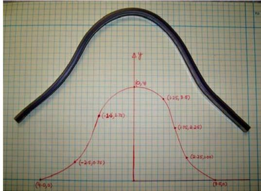
Figure 1. Using a flexible curve to draw a curve of known length. This is only a sample curve. Your curve may look different, have different co-ordinates, and /or have different number of points chosen (errata – the first co-ordinate in the figure is  $(-4,0)$ ).
